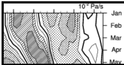
Figure 5g: Example of a special contour effect. This plot uses the resource gsnZeroLineContourThicknessF to make the zero line thicker, and then uses various contour fill patterns to shade different areas.
